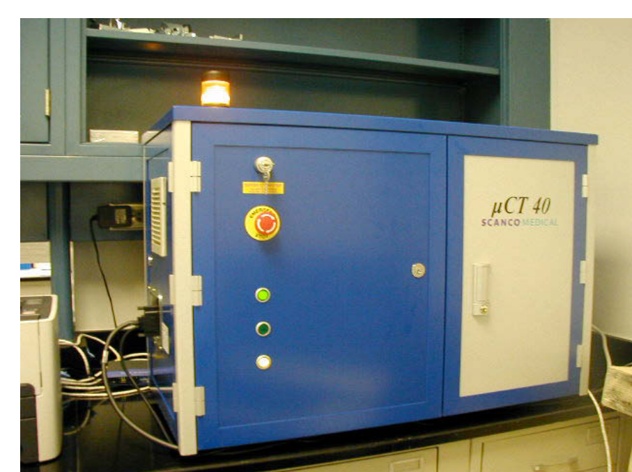
Desktop Microtomographic imaging system (µCT40.scanco Medical AG, Bassersdorf, Switzerland)
