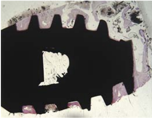
Fig. 1. Midline nondecalcified thin section image of a plateau design root from implant retrieved after 60 months in vivo with a BIC of 52%.
